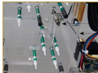
Top contacting with screwing unit (SBE)
