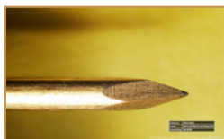
Test probe tip after 5 penetration cycles
