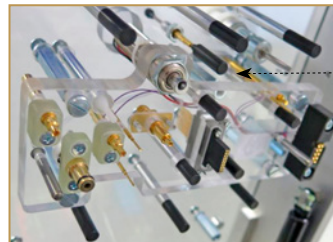
Top contacting with button activator (TAB)
