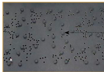
moving plate with PCB support pins (PAS)
