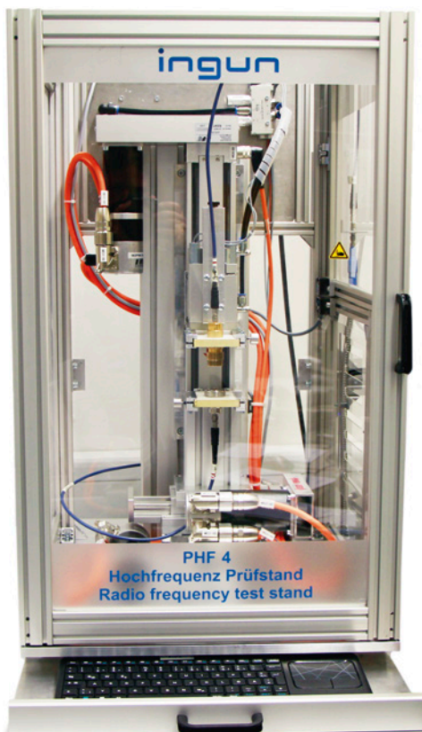
RF endurance test stand PHF4 performs a combination of mechanical and electrical life cycle tests
