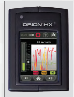
Histogram graph displays history of harmonic response and power adjustment from 10 - 60 second duration.
