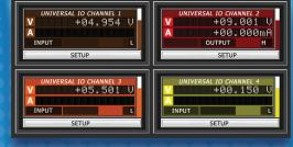
8 fully programmable, independent channels ±10V OUT @20mA, ±15V IN 5 logic presets available
